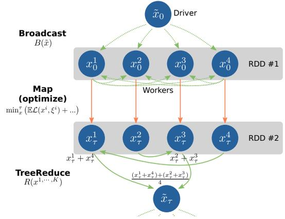
Fig. 4. Synchronous data-parallel training in SparkNet.
