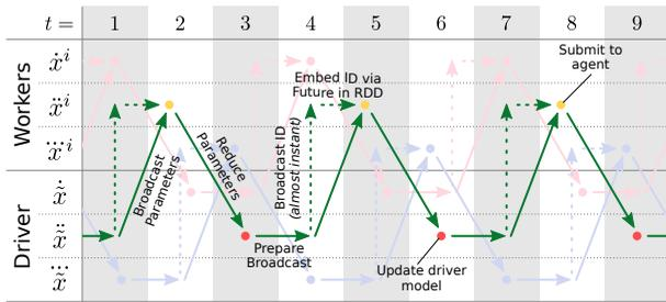
Fig. 12. Data flow of model updates in MPCA SGD to allow executing broadcast and reduce in parallel. The highlighted path represents the parameter exchange cycle for the second model shard ( $\hat{x}$ ).
