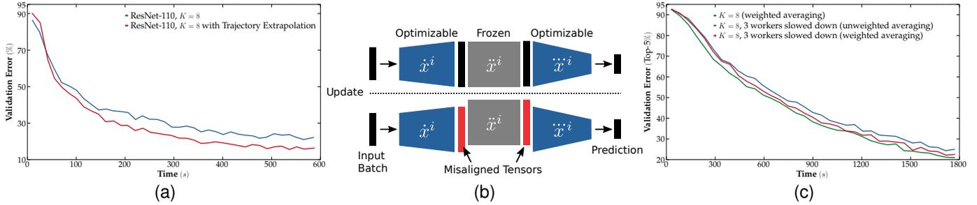
Fig. 10. (a) Influence of linearly extrapolating the joint model on the prediction error; (b) Tensor misalignment upon separately updating a model shard; (c) Influence of stragglers on the prediction error if reduction is done via unweighted averaging, compared to weighted averaging using  $\tau^i$ .
