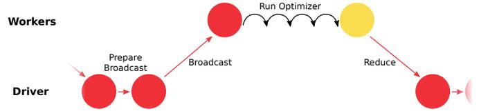
Fig. 1. Classic synchronous approach for decentrally training deep learning models (●) using MapReduce. After broadcasting each worker starts optimizing its local model replica and independently computes updated model parameters (●) that are then aggregated during reduction to form the starting state for the next optimization cycle. Note how communication and computation phases are interleaved.
