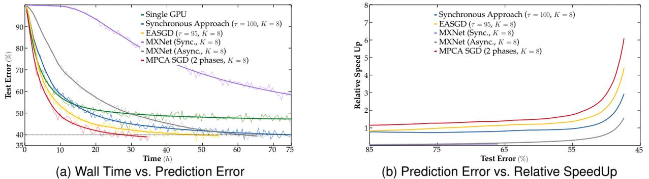
Fig. 15. Comparison of convergence performance for a VGG-A on the full ImageNet-1k dataset.
