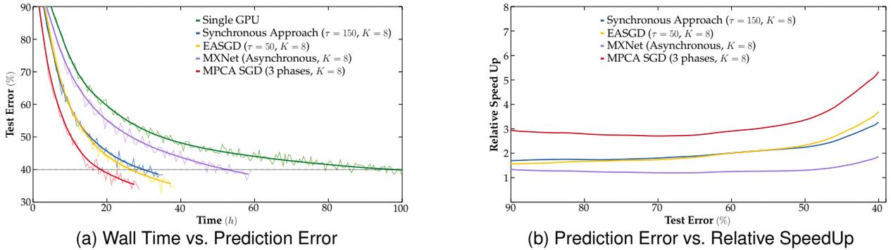
Fig. 14. Comparison of convergence performance for a ResNet-152 on the full ImageNet-1k dataset.
