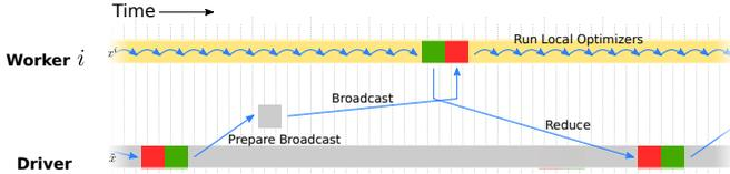
Fig. 6. Single phase coordinated asynchronous communication pattern. The cluster is either exclusively broadcasting or reducing. Because the network bandwidth is poorly utilized, isolated learning phases are very long. However, note how model training is only briefly interrupted in comparison to the significant stalling of the synchronous approach (Fig. 5).
